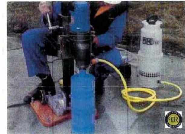
4" cores taken to truly validate results through Microviscosity and Penetration Values
