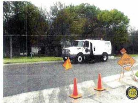
We follow up with our Regenerative air sweeper to ensure a clean roadway free of any residual sand and debris to complete our Rejuvenation process
