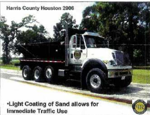
Using clean, washed concrete sand, we apply a light coating to the road to address any skid resistance issues, tracking onto vehicles or driveways and ensure minimal disruption to traffic and residents
