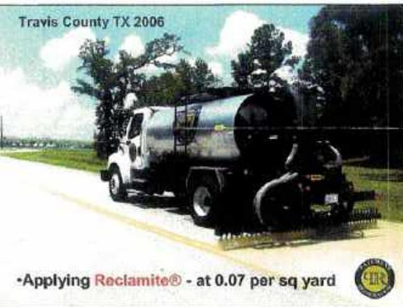
Our latest Rosco distributor trucks apply an accurate computer controlled spread for even applications for full road coverage curb to curb. Smaller hard to reach Hot Spots are dealt with our mobile ATV sprayer
