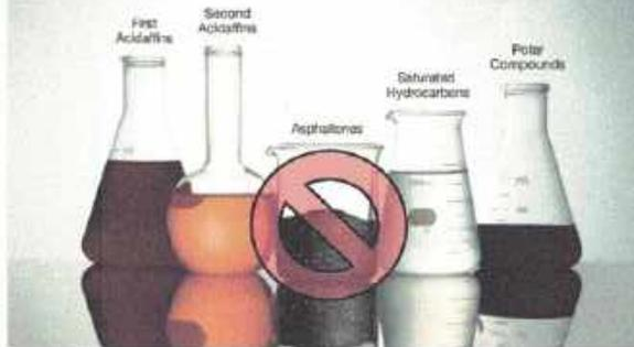
Because **Reclamite®** does not include the asphaltenes component, the product is able to fully penetrate the asphalt surface. This process restores the chemical maltene balance lost due to oxidation and other natural degradation.
